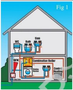
When a combi-boiler is used, and there is no hot water cylinder, a single Water-King unit fitted on the rising main will provide the whole house with protection. If only the boiler needs protection from scale, locate the Water-King within 2 meters of it. This also applies to a hot water cylinder under mains pressure.
